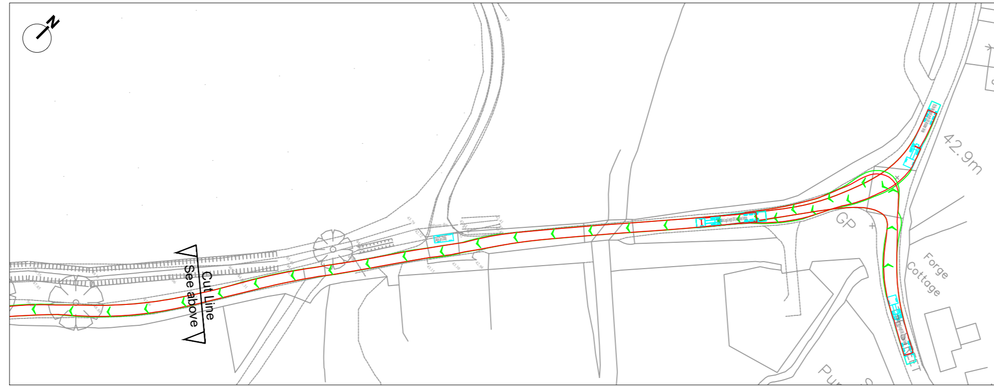
Swept Path Analysis of a 18.55m Articulated Vehicle Travelling Towards Site Access from B1066
